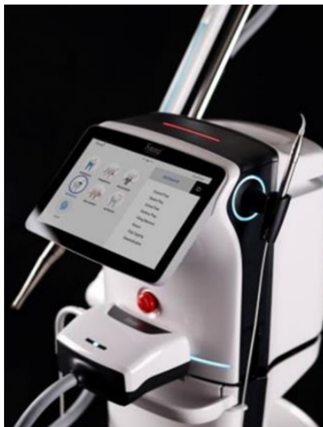
Fig. 7: The Er:YAG laser system of SkyPulse. The laser system includes the two most recent laser-assisted irrigation modalities, SSP and SWEEPS, allowing for a full SSP/SWEEPS endodontic treatment.
