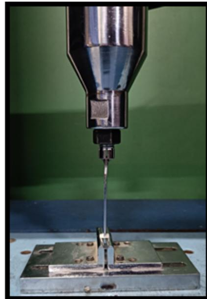
**Figure 9:** Two point test with universal testing machine (cross head speed: 1mm/min Distance support: 7mm)
